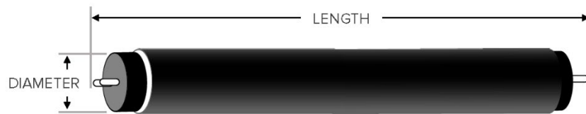
994 Figure 1: Dimensions of linear replacement lamps to be reported on the application form.
