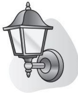
Figure 11: Example of a non-eligible outdoor uplight-emitting wall-mounted area luminaire. (Image credit: Focus on Energy®)
