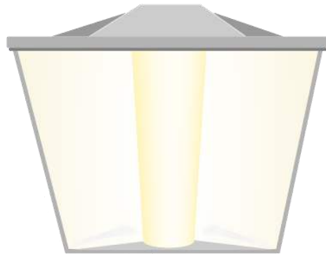
Figure 4: Isometric view of a troffer with a luminous basket and luminous panels on each side. The luminous shape would be represented by a rectangular object with luminous sides encompassing the entire luminaire.
