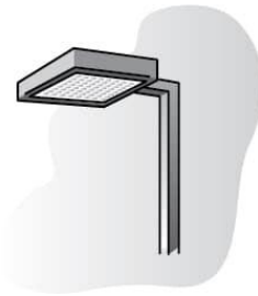
Figure 5: Example of an outdoor pole/arm-mounted area and roadway luminaire. (Image credit: Focus on Energy®)
