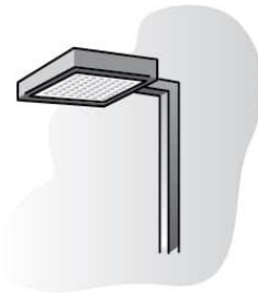
Figure 36: Example of an outdoor pole/arm-mounted area and roadway luminaire. (Image credit: Focus on Energy®)
