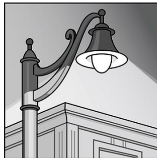
Figure 6: Example of an outdoor pole/arm-mounted decorative luminaire. (Image credit: Efficiency Vermont)
