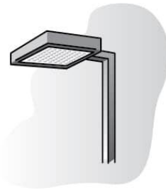
Figure 34: Example of an outdoor pole/arm-mounted area and roadway luminaire. (Image credit: Focus on Energy®)
