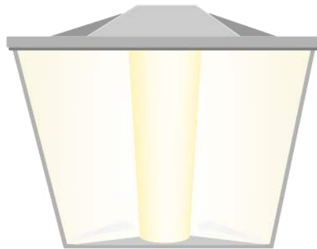
Figure 4: Isometric view of a troffer with a luminous basket and luminous panels on each side. The luminous shape would be represented by a rectangle or rectangle with luminous sides encompassing the entire luminaire.
