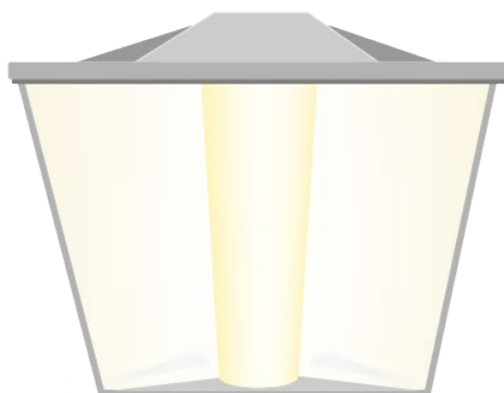
Figure 3: Isometric view of a troffer with a luminous basket and luminous panels on each side. The luminous shape would be represented by a rectangle or rectangle with luminous sides encompassing entire luminaire.
