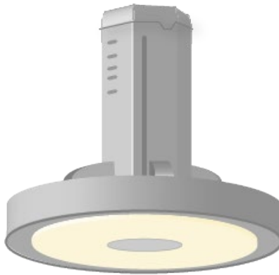
Figure 5: Isometric view of a high bay product with LEDs on the underside. The luminous shape would be represented by a 2D luminous circle, with length and width elements represented as negative values of the respective diameter (see LM-63 for details). If the luminous surfaces were on the sides as well, a vertical cylinder or rectangle with luminous sides would be used instead.
